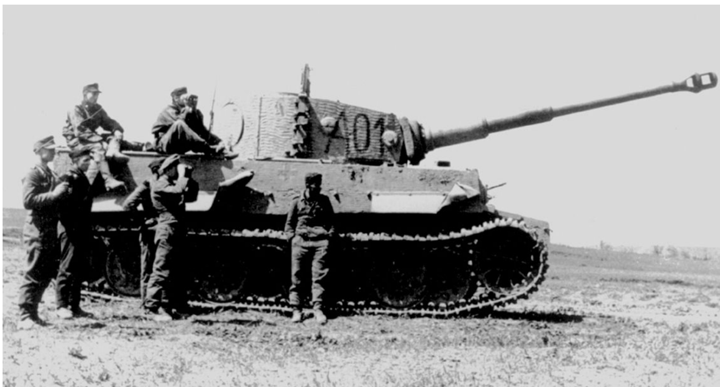
A late production Tiger with the all-steel wheels that were introduced in January 1944.
