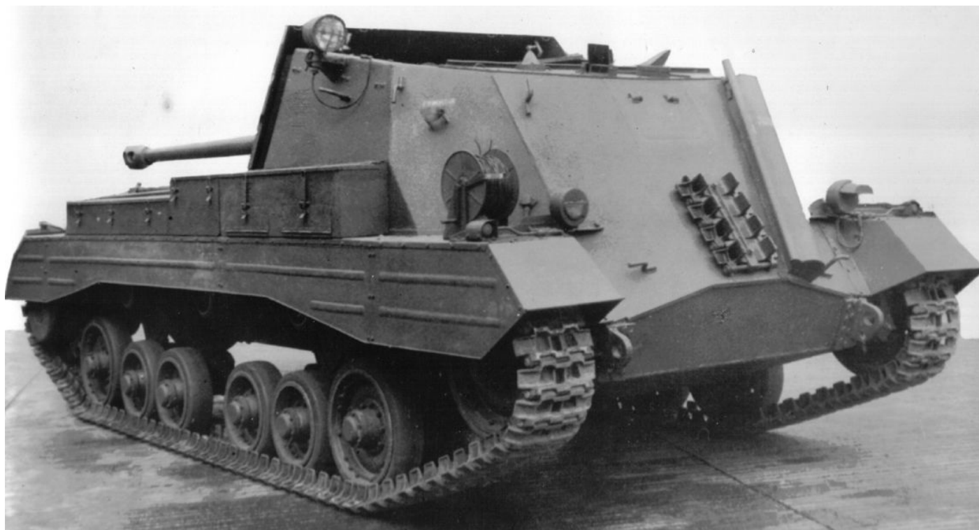
This unsatisfactory interim Tiger killer is the Archer, which married the 17-pounder gun with the Valentine tank chassis and joined the British Army in October 1944. The gun faced to the rear of the vehicle.
