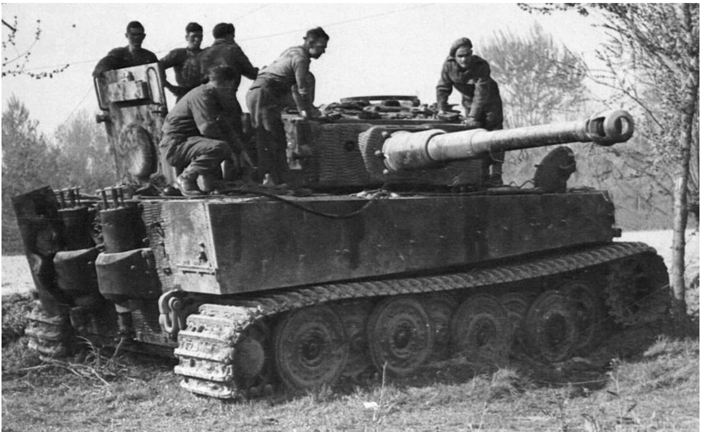
British or Canadian troops examining a late production Tiger, identifiable by its steel road wheels, in Normandy. This particular vehicle has lost its track guards.
