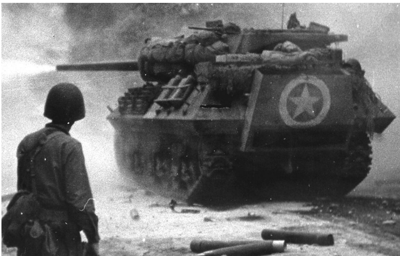
The M10 Gun Motor Carriage was armed with the 3in M7 gun that could tackle a Tiger, but it lacked adequate armour, like the Firefly.
