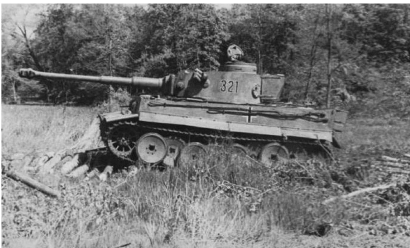
An early Tiger negotiating a log road. Despite the wide off-road tracks, the tank's weight could be a problem on soft ground.
