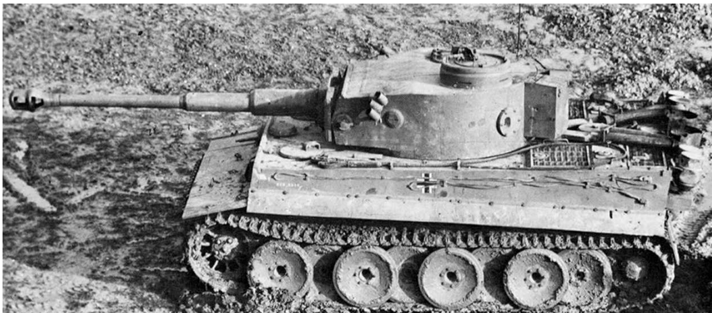
A side view of an early production Tiger I. Note the cylindrical cupola with vision slits, the machine-pistol port at the rear of the turret by the storage bin, and the distinctive rubber-rimmed dish-shaped road wheels.
