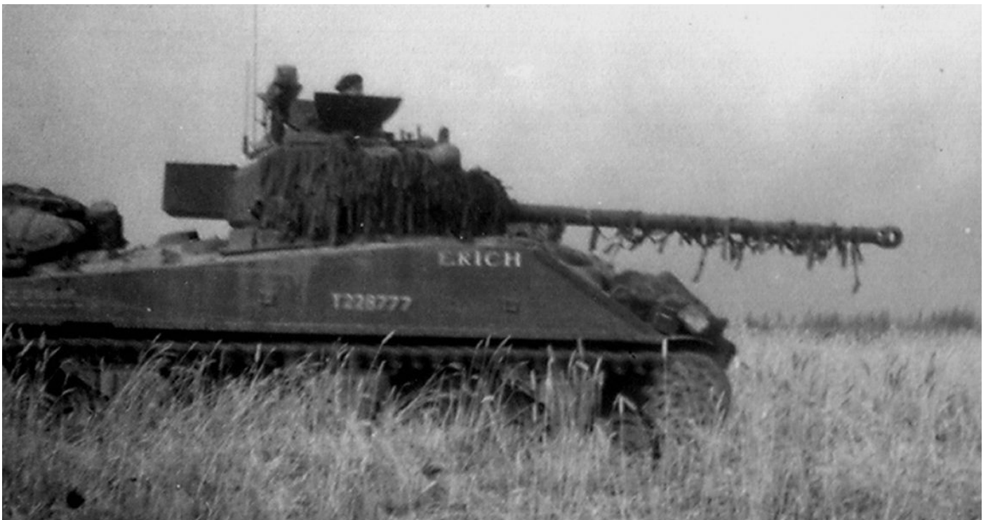
The one tank capable of taking on the Tiger was the Sherman Firefly, armed with the British 17-pounder anti-tank gun.
