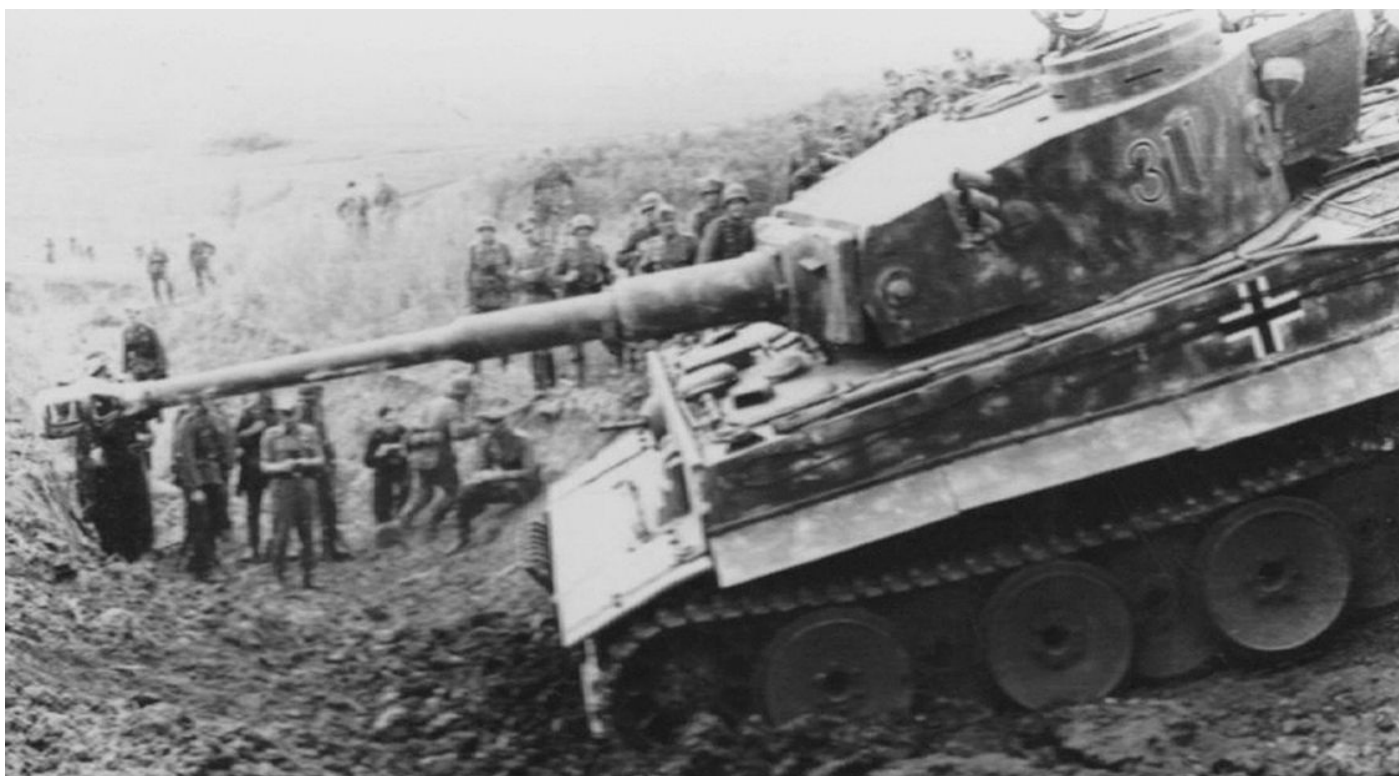
An early production Tiger I on the Eastern Front. Despite its wide tracks, the mud and ice often caused problems with the complicated overlapping road wheels.
