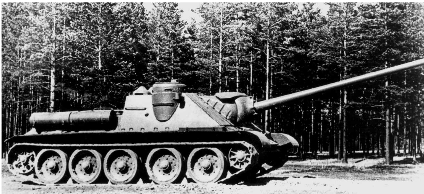
Soviet attempts to counter the Tiger included the SU-85/100 tank-destroyer, which married an 85mm/100mm gun to the T-34 chassis respectively.
