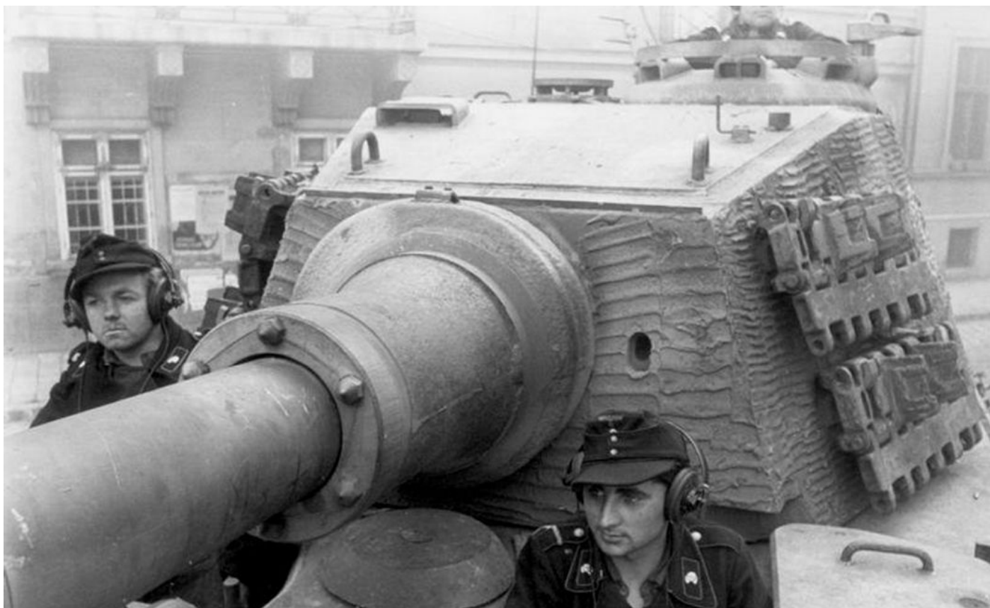
A close-up of the very large mantlet on the improved Henschel/Wegmann turret.
