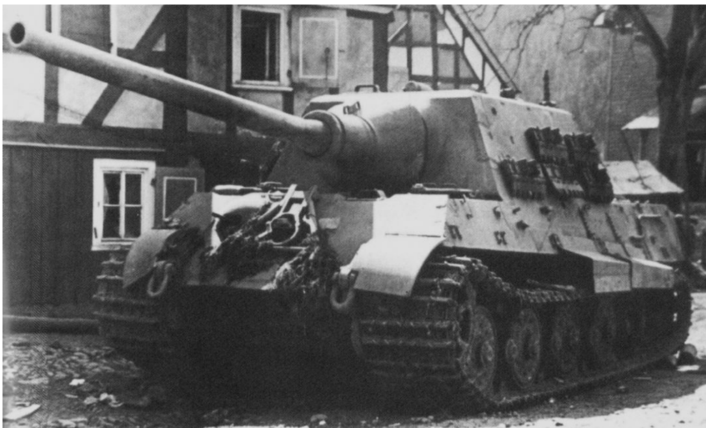
Two views of the Jagdtiger found in Obernetphen, Germany, in April 1945. The enormous 128mm gun gave the Jagdtiger great killing power but little else.
