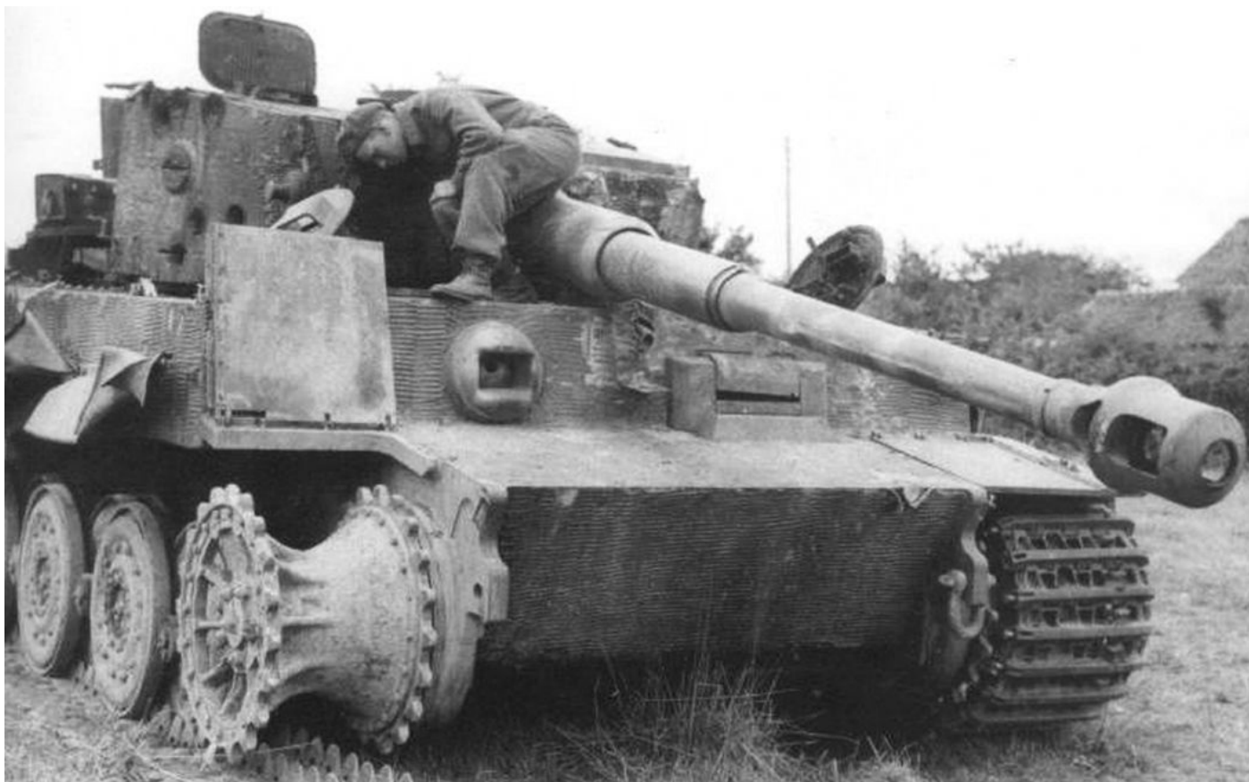
Another late production model getting the once-over in Normandy. The corrugated surface on this tank (and the previous one) is due to the Zimmerit paste that was applied from 1943 onwards to prevent the attaching of magnetic anti-tank hollow charges.
