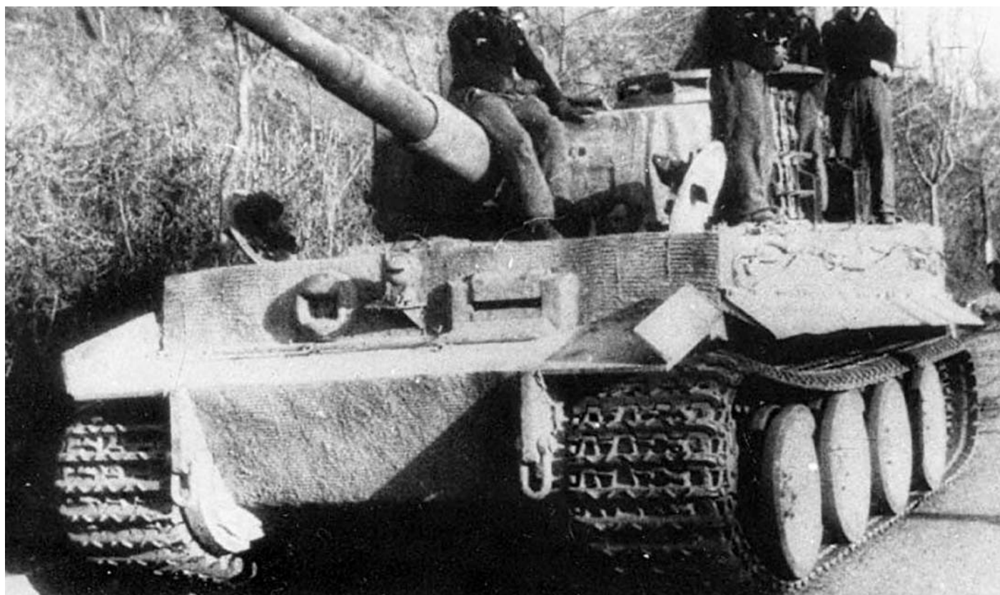
A mid-production Tiger coated in Zimmerit paste.
