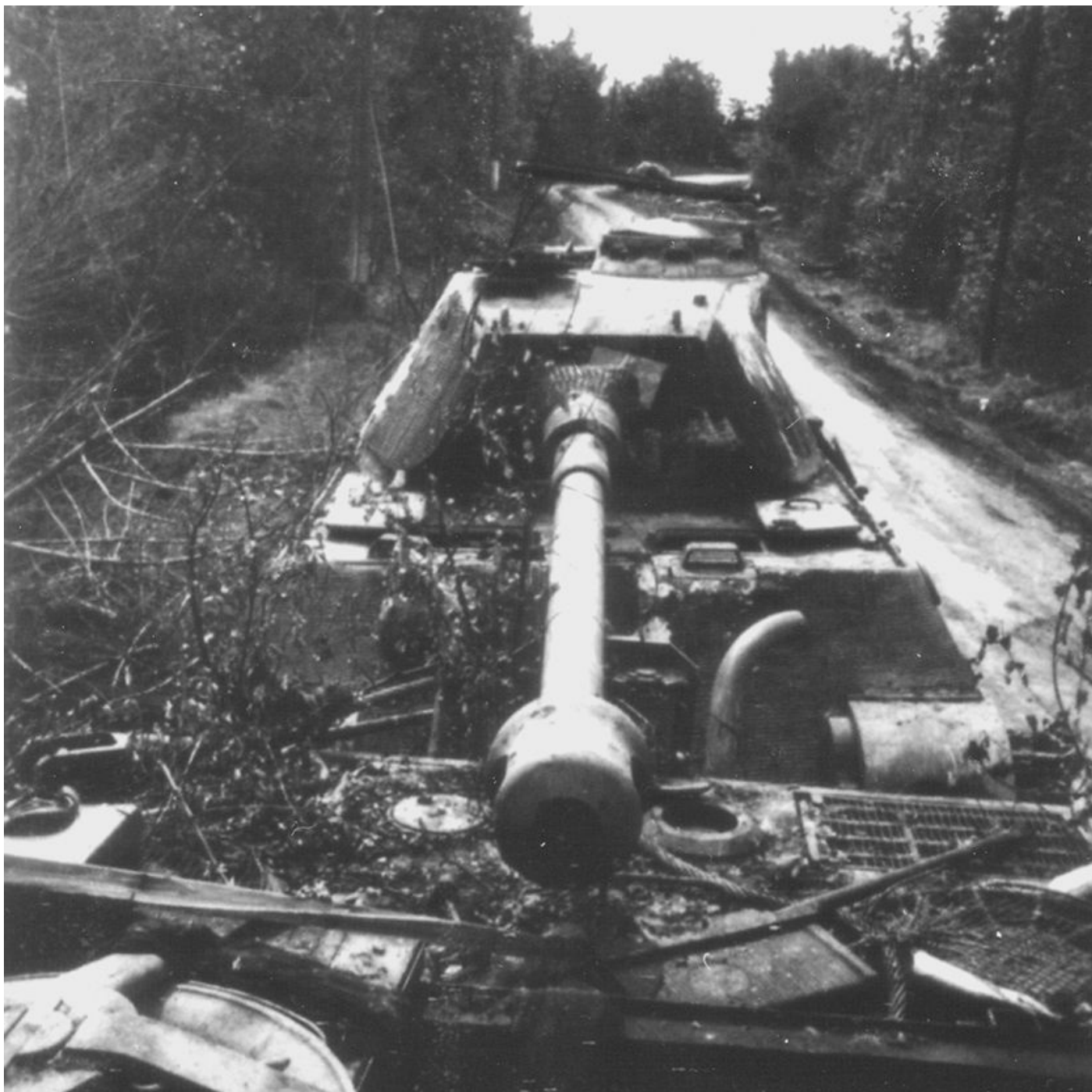
A frontal view showing the curve of the Porsche turret. The tank in front of it is a Bergepanther recovery vehicle.
