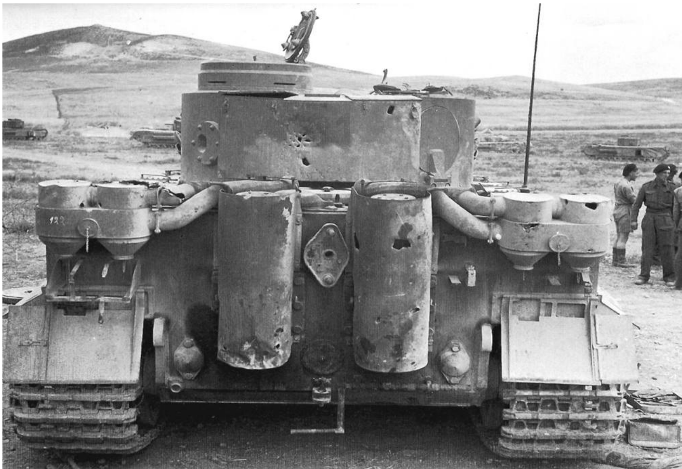
The rear end of an early production Tiger I captured in Tunisia by the British Army. Clearly visible are the massive exhausts and the Feifel air cleaner system on either side. The turret escape hatch on the right was installed from December 1942 onwards.
