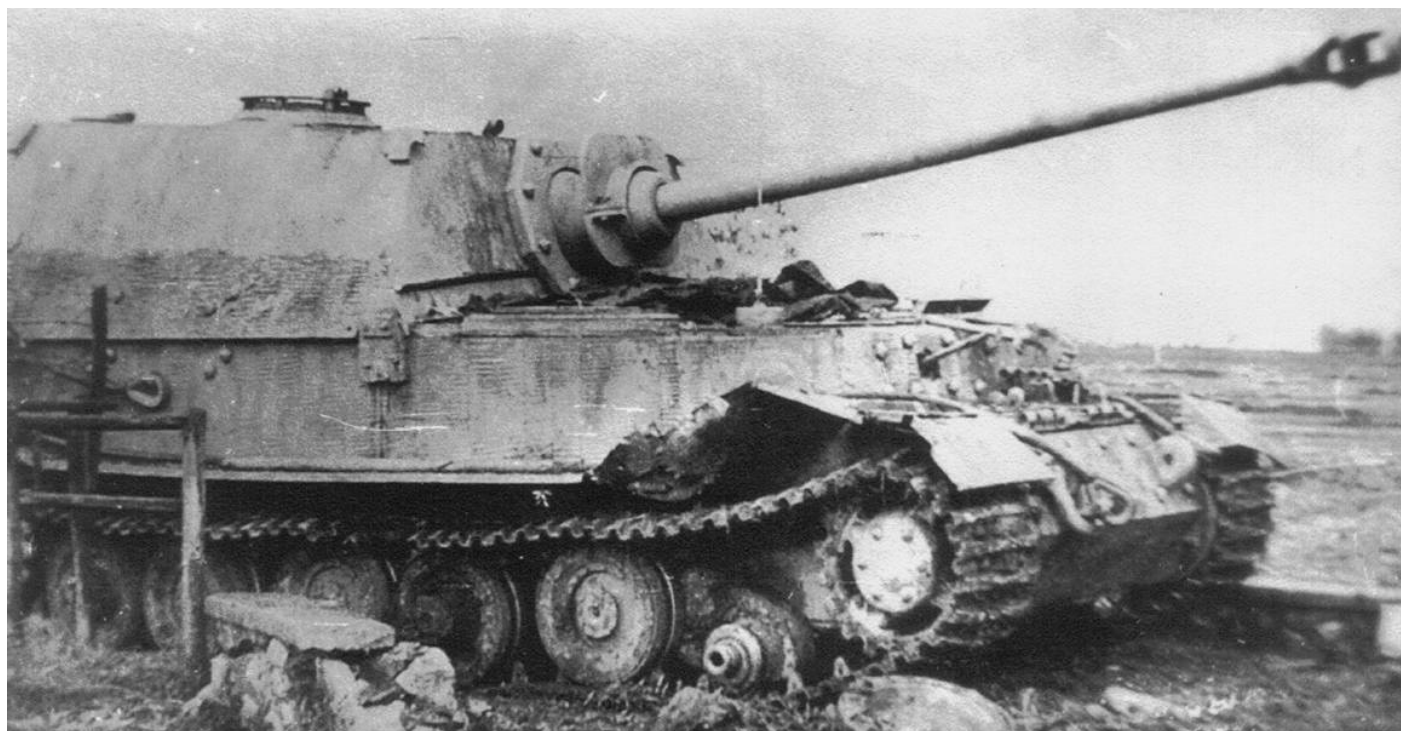
Even the half-hearted improvements that converted the Ferdinand into the Elefant did little to remedy its shortcomings. This is the rebuilt model with added hull machine gun and commander's cupola.
