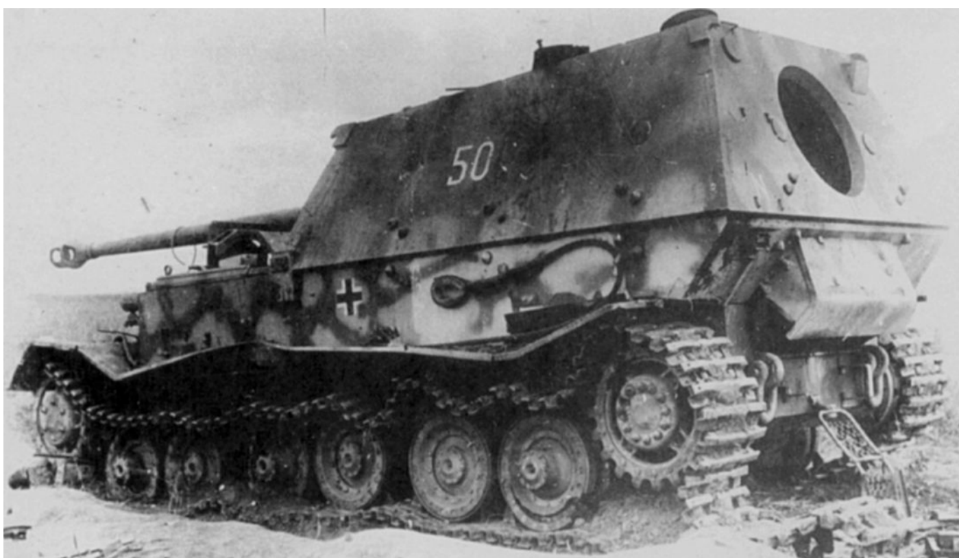
This Ferdinand seems to have fallen prey to mines that have severed the track and damaged the road wheels. (It may be the same vehicle as that shown on pp. 50 and 141 .)
