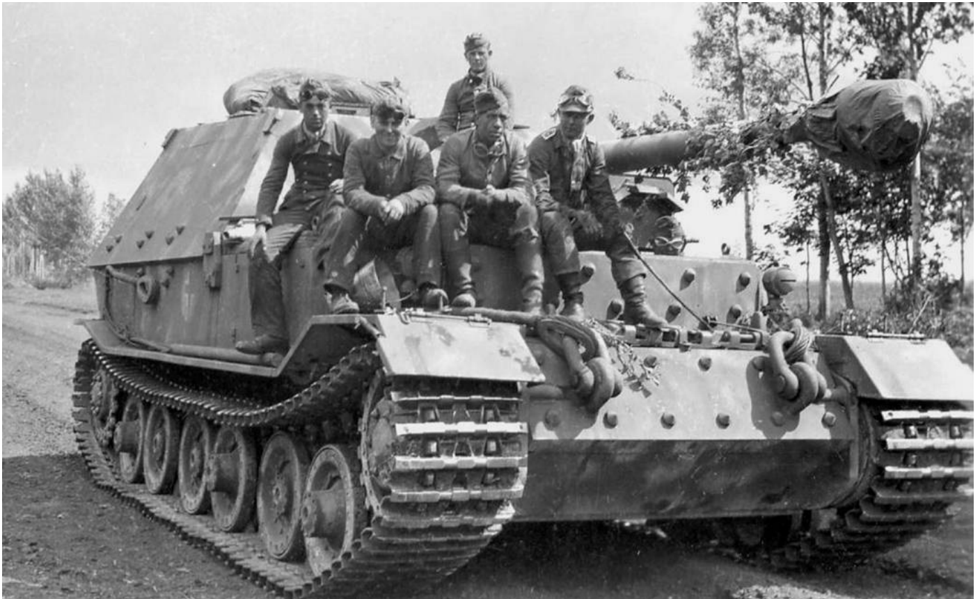
In theory the Ferdinand tank-destroyer was a good use for the rejected Porsche Tiger I chassis.
