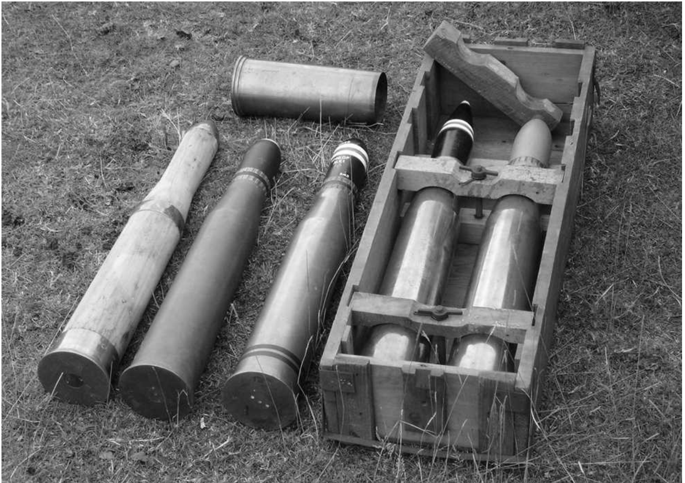
A selection of 17-pounder ammunition, giving some impression of the size of the rounds. On the left is a wooden drill round.
