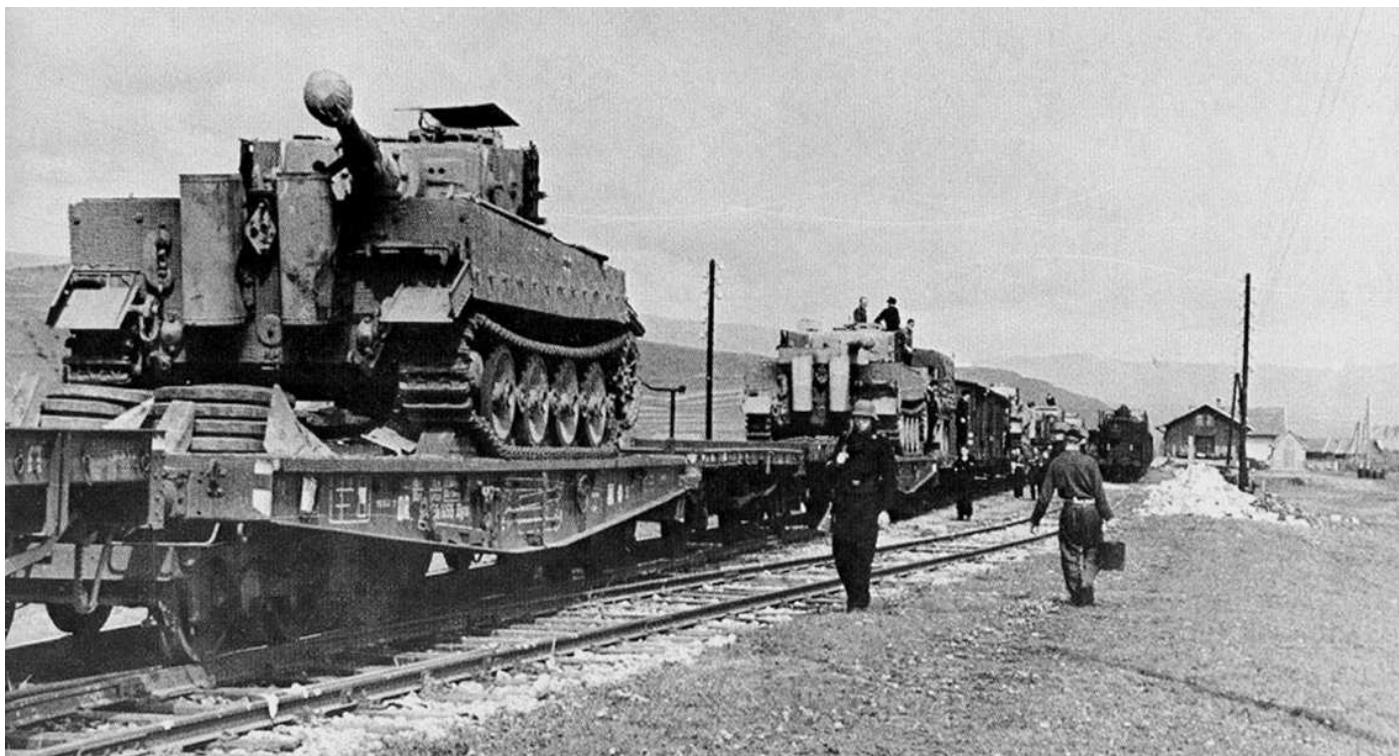
This mid-production Tiger is fitted with its narrow road tracks, to accommodate which the outer row of road wheels has been removed and stacked behind the tank.
