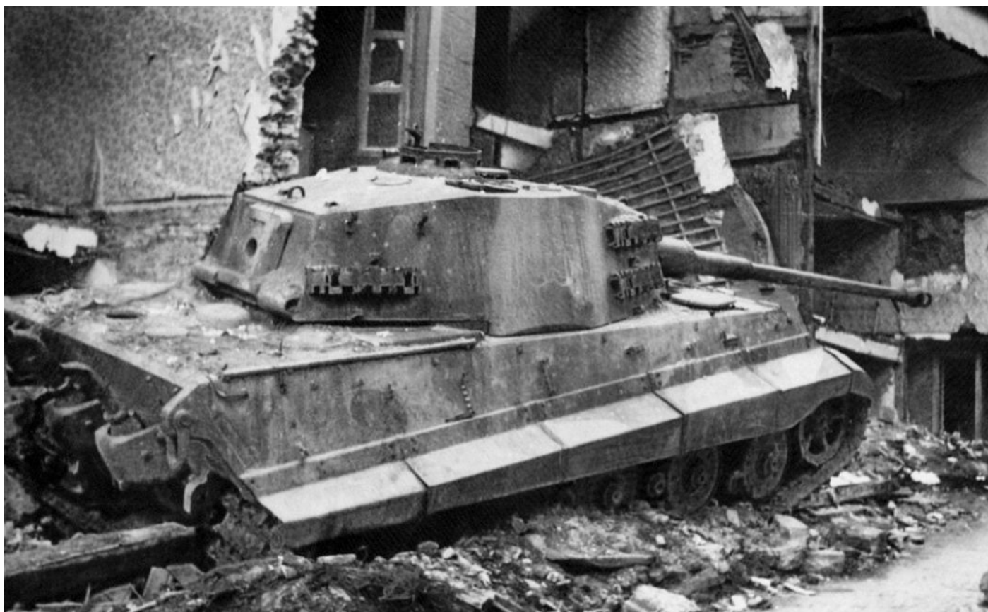
Two views of a Tiger II knocked out during the Ardennes offensive. Note the distinctive camouflage applied to the hull, track guards and turret. Track links have been placed on the turret to enhance the armour.
