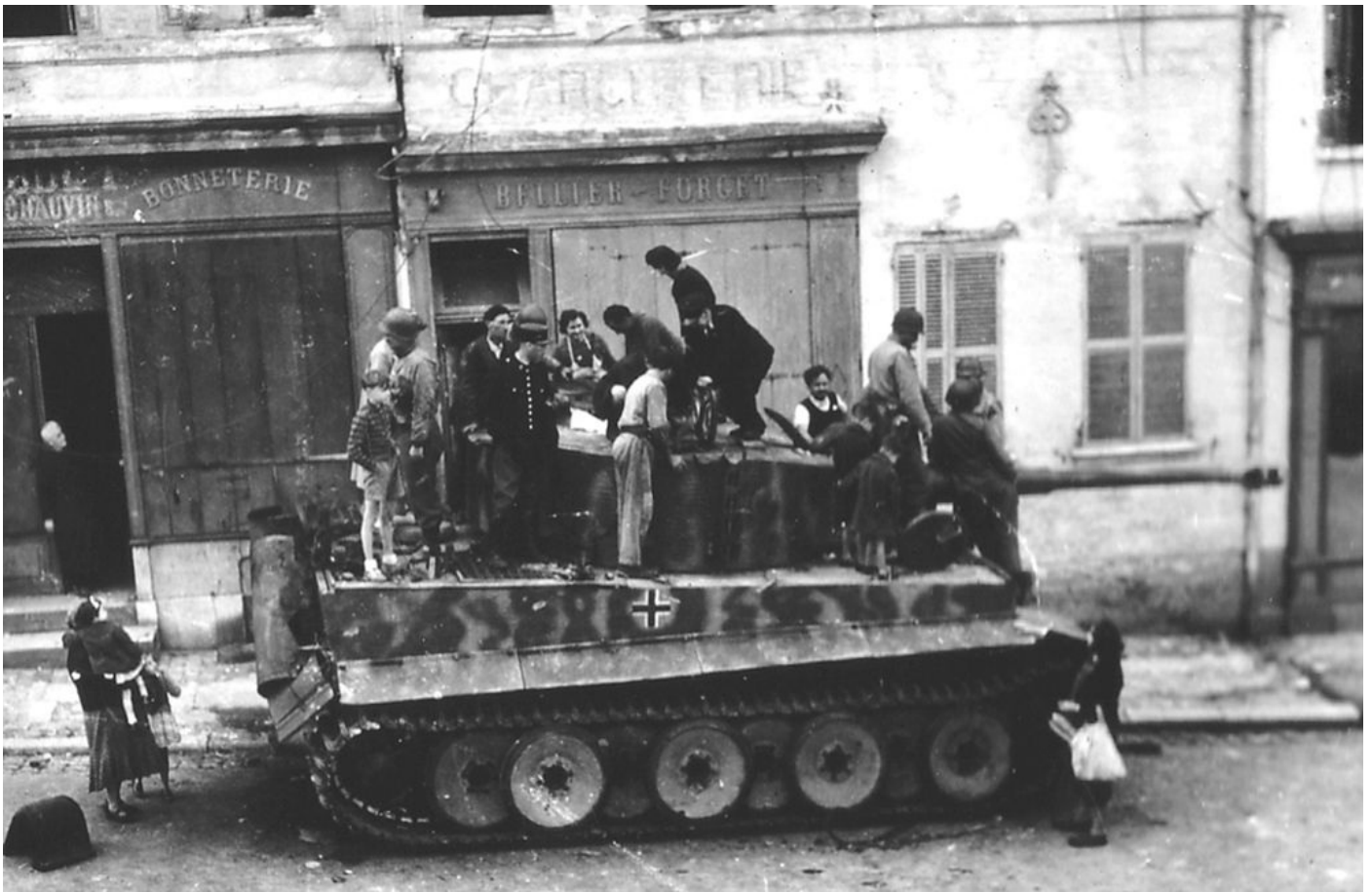
This mid-production Tiger I was abandoned in Normandy in 1944. It retained the rubber-rimmed road wheels but had a smaller cupola with periscopes. The air cleaning system had been dispensed with by this stage.
