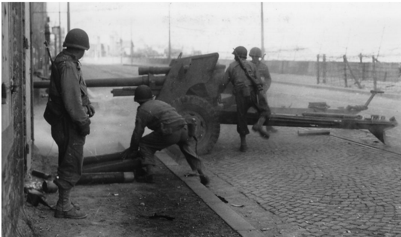
The American M5 3in (76.2mm) anti-tank gun was the only towed weapon bigger than the standard 57mm anti-tank gun. It was also installed in the M10 tank-destroyer.
