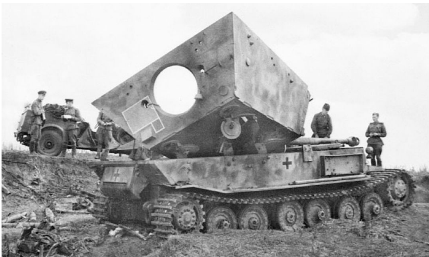
This Ferdinand suffered such a massive internal explosion that its superstructure was torn off the chassis, flipped over and dropped down again.
